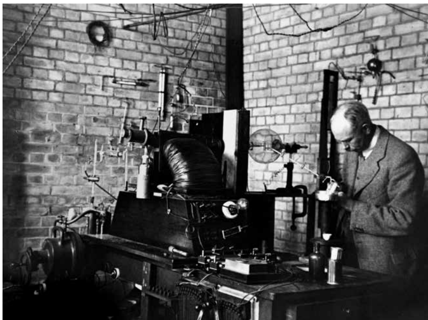
Aston at work on his mass spectrometer (Copyright Cavendish Laboratory)
